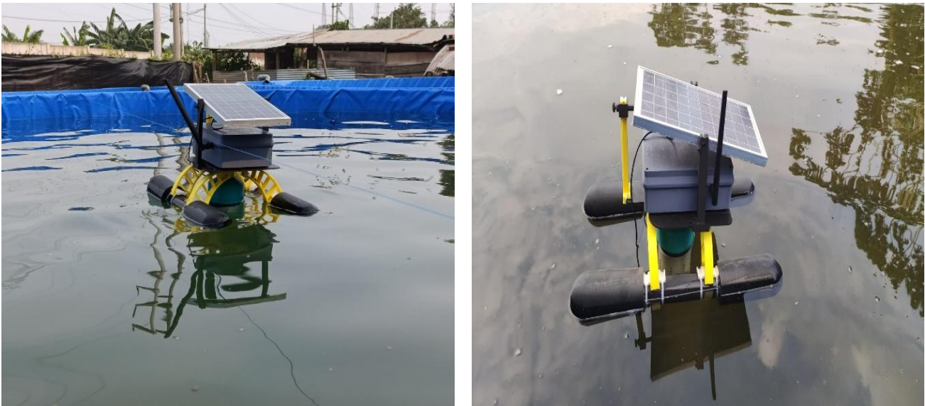
Figure 6. Testing of the buoy prototype in a real aquatic environment
